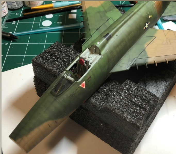
18) Not a great pic but here is the final effect. Once this is done I spray Model Master flat to seal everything. Model Master flat is dead flat and really tones all the weathering down. If you are too subtle in your weathering application you can lose the effects under this dead flat coat.
